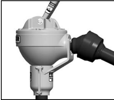
FIG. 8 - AUGER ADAPTER GUARD INSTALLED
